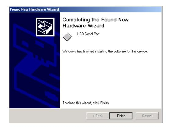
You can check the Com port number of the Sapphire from Device Manager. It is COM3 in this example.
